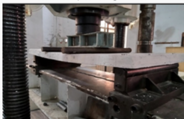
Flexure Testing of a Specimen on Shimadzu UTM
