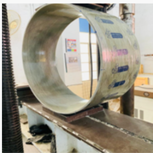
Parallel Plate Load Test
