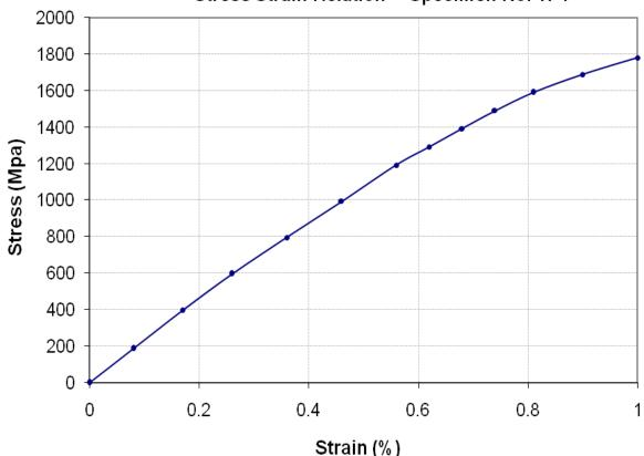
Stress Strain Relation -- Specimen No. W 1
